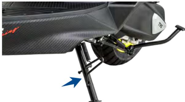
Side stand can be operated by sitting on vehicle with your left foot by pushing it away from the vehicle till it stops.
