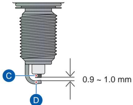
After cleaning and inspecting the gap, reinstall the spark plug and tighten by hand to avoid cross threading. Finally tighten using spark plug spanner. Do not over tight or cross thread the spark plug.
