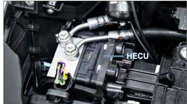
As soon as the actual circumstances arises, the system reacts instantly and adjusts braking force accordingly to achieve optimum braking.
