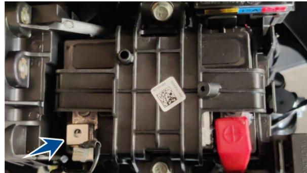
4. While connecting the terminals observe the correct polarity. Connect the red wire to the positive (+) terminal and the black wire to the negative terminal (-) of the battery.
