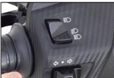
The same pass-by switch is used to operate head lamp low / high beam continuous glowing.
