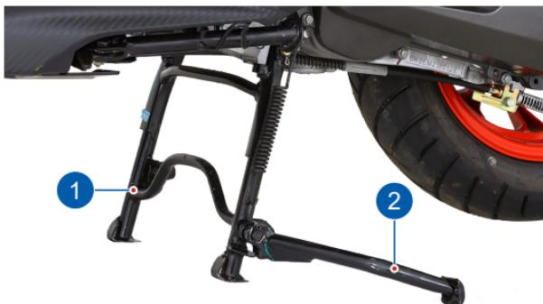
To place the vehicle on centre stand, hold the handle bar left grip with left hand, place your foot firmly on the centre stand extension (2) while ensuring that both the stand shoes are touching the ground, press the stand extension.
