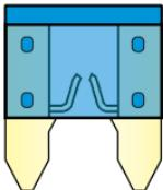
5. Inspect the fuse for failure. If found defective Replace the blown fuse with a new (extra fuses are provided in the wiring harness itself in a pouch).
