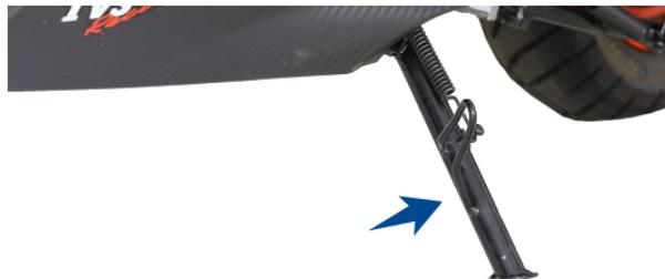
Side stand can be operated by sitting on vehicle with your left foot by pushing it away from the vehicle till it stops.
