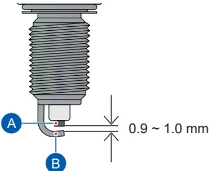
After cleaning and inspecting the gap, reinstall the spark plug and tighten by hand to avoid cross threading. Finally tighten using spark plug spanner. Do not over tight or cross thread the spark plug.
