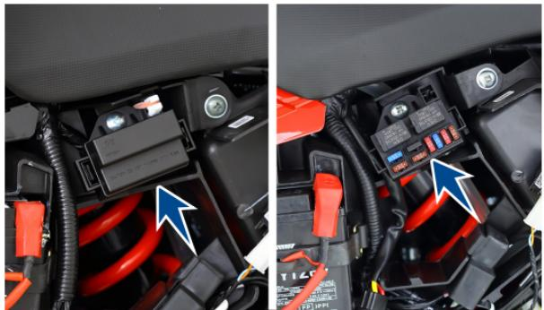
3. Replace the blown fuse with a new one with same rating (extra fuses are provided inside the fuse case itself).
