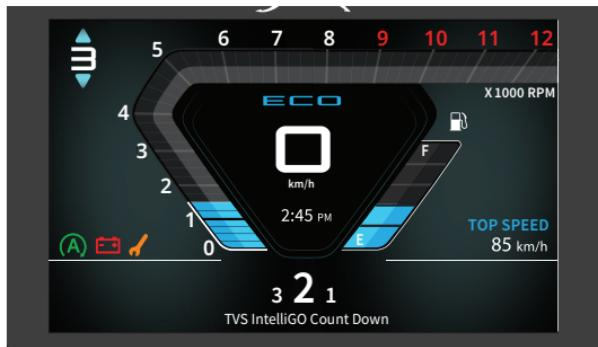
Now, the intelliGO indicator again starts glowing continually during the engine stop to indicate that the vehicle has stopped due to 'intelliGO' system.
