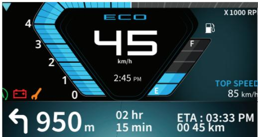
On reaching the destination, the instrument cluster displays the arrival of destination as shown:
