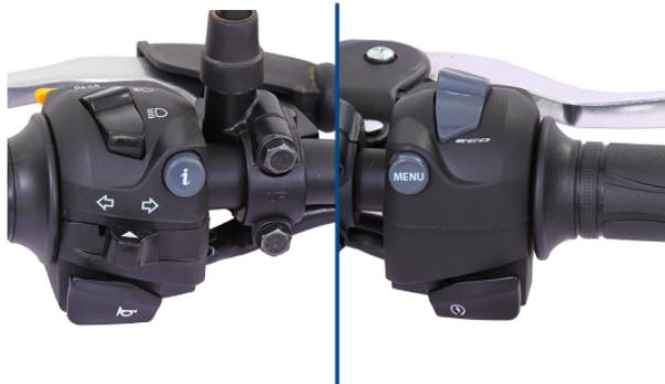
'Menu switch' is located at the right side of the handle bar. 'Menu switch' is used to access the connected instrument cluster's display to various options like Trip A, Trip B, Range, Average mileage, Average speed and top speed.
