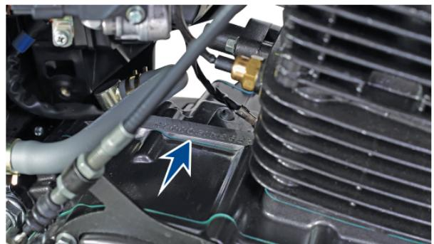
Engine serial number is stamped on the top surface of the left side crankcase assembly near the cylinder block.
