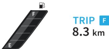
If the fuel level remains in minimum safe level, the reading is saved even after the ignition 'OFF'. The count stops and clears automatically after a certain distance of run with the fuel level above minimum safe level.
