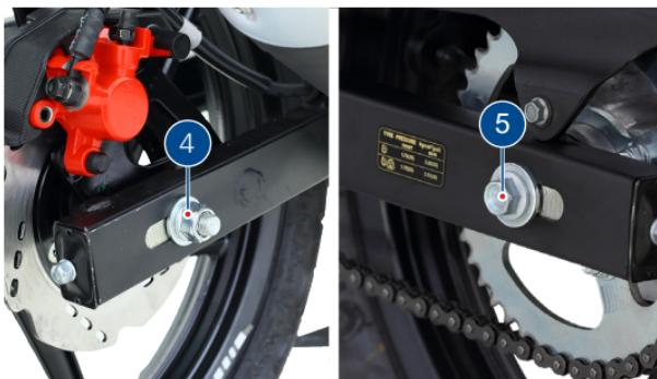
5. Re-assemble the other parts in the reverse order of removal. During re-assembly, engage the drum sprocket with the wheel along with the drive chain and then assemble the wheel into swing arm.
