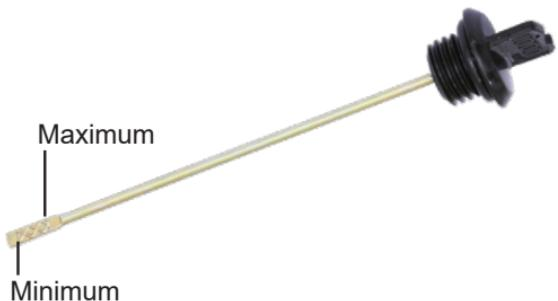
6. If the oil level is less than the minimum level, add TVS TRU4 PREMIUM oil ((SAE 10W30 API-SL JASO MA2) upto the maximum level mark.
