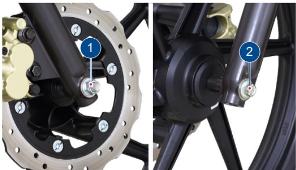
3. In case of disc brake model, remove the spacers from both side of the wheel. In drum brake model remove a spacer from right side of the wheel.
