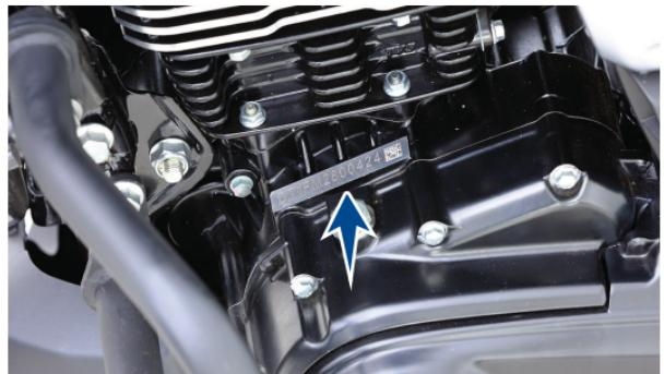
Engine serial number is engraved on the left side crankcase assembly near cylinder block as shown.
