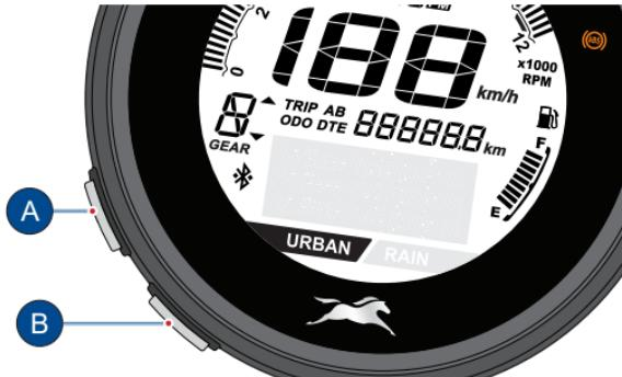
The 'Mode' (A) and 'Set' (B) buttons are provided to change between various modes and to set some of the digital display functions of the instrument cluster. The sequence of modes and their selections are explained in detail below.
