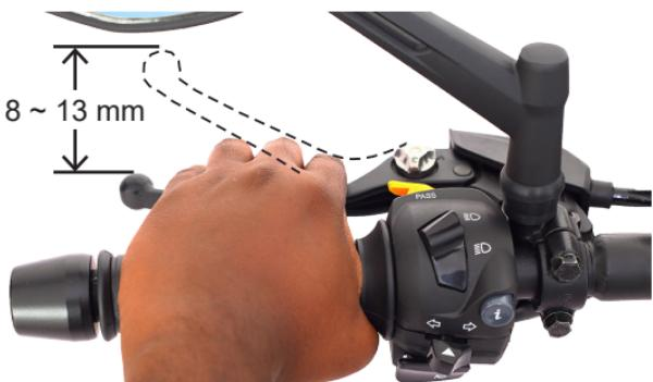
2. Loosen the lock nut (2) while holding the clutch cable adjusting nut (1). Adjust the clutch cable adjusting nut (1) 'in' or 'out' to give sufficient play in the clutch lever.
