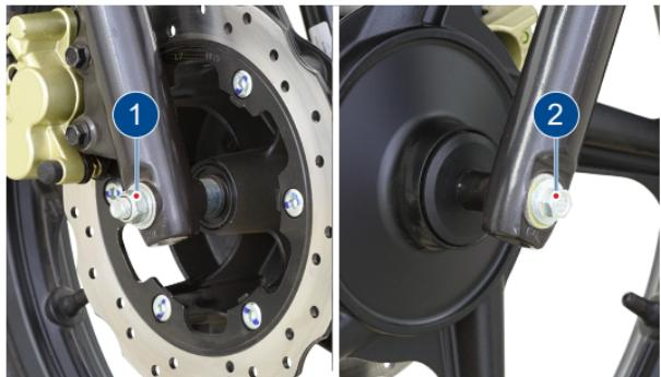
4. Incase of drum brake model, remove a spacer from right side of the wheel.
