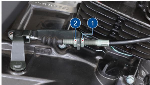
2. Loosen the lock nut (2) while holding the clutch cable adjusting nut (1).
