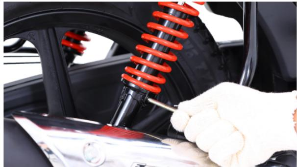
If the spring is adjusted to maximum notch, then it will be stiffer which is good for heavy loads.
