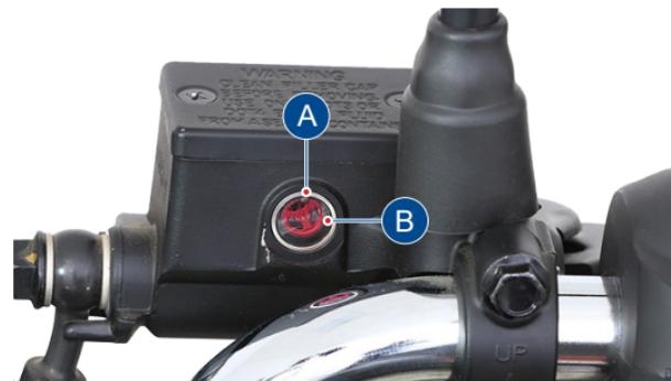
1. Check the master cylinder brake fluid level through the view piece glass (A).
