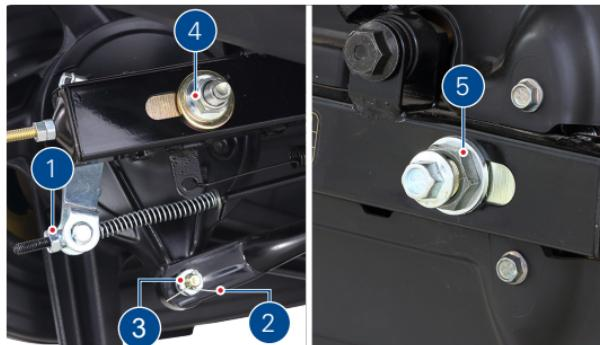
6. For locating and reassembling the rear wheel easily, engage the gear. This will arrest the free movement of the drum sprocket.
