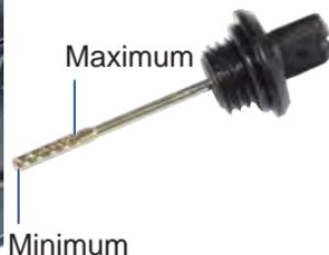
6. If the oil level is less than the minimum level, add 'TVS TRU4 PREMIUM oil (SAE 10W30 API-SL, JASO MA2)' upto the maximum level mark.
