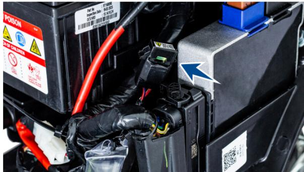
5. Replace the blown fuse with a new (extra fuse is provided in the wiring harness itself in a pouch).
