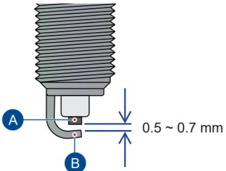
Inspect the spark plug gap with a wire gauge / feeler gauge. Readjust the spark plug gap to **0.5 ~ 0.7 mm** if required.
