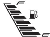
All the six bars will be displayed when the fuel in the tank reaches above 5 liters approximately (full tank). When the fuel reaches half tank (3.2 liters approx.) the fuel gauge displays only three bars as shown.
