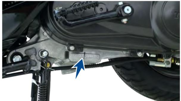
The engine serial number is stamped on the left side of the engine, at the bottom, near center stand mounting. See bottom to read serial number.
