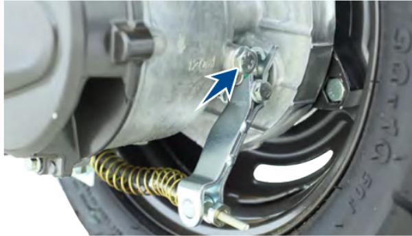
6. Reassemble the oil level bolt with new fiber washer.
