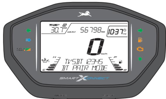
5. The connected instrument cluster's Bluetooth name is prefixed by TVSBT and followed by alpha-numeric digits. Ex : 'TVSBT12345'. This Bluetooth name can be found by changing the cluster mode into BT pair mode.
