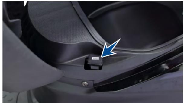
5. Turn 'ON' the ignition lock and check for proper functioning of electrical systems. Incase the fuse fails again, consult the nearest TVS Motor Company Authorised Main Dealer / Authorised Dealer.
