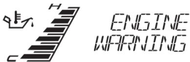
On occurrence of the above error message, the vehicle should be kept in idling for 10 minutes approx. and switch 'OFF' the vehicle. If the problem continues even after cooling the engine, take the vehicle to TVS Motor Company Authorised Main Dealer or Authorised Dealer and get it rectified.
