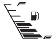
When the fuel reaches minimum safe level (1.2 liters approx.), the last bar of the fuel gauge starts blinking and low fuel indicator starts glowing.
