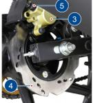
3. If the brake fluid level is below minimum or while applying brake if you feel the brake is more spongy or ineffective due to air entry, contact TVS Motor Company Authorised Main Dealer / Authorised Dealer for topping-up the brake fluid, air bleeding and other brake related inspections.
