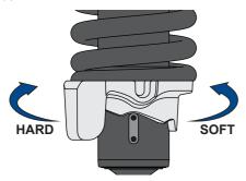
Adjust the spring pre-load by shifting the adjuster to the required notch according to the different load conditions. The more you compress the spring, the suspension becomes more stiff.
