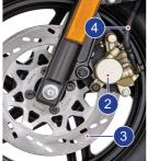
5. If the brake fluid level is below the 'MIN' mark or while applying brake if you feel the brake is more spongy or ineffective due to air entry and if any rattling play is observed in both the brake levers, contact TVS Motor Company Authorised Main Dealer or Authorised Dealer for topping-up the brake fluid, air bleeding and other brake related inspections.
