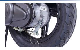
Turn the adjuster nut in clockwise direction for reducing free play or in anti-clockwise direction for increasing the free play.
