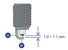
After cleaning and adjusting the gap, reinstall the spark plug and tighten by hand to avoid cross threading. Finally tighten using spark plug spanner.
