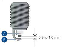
Inspect the spark plug gap with a wire gauge / feeler gauge. Readjust the spark plug gap to  $0.9 \sim 1.0$  mm if the gap is found more.
