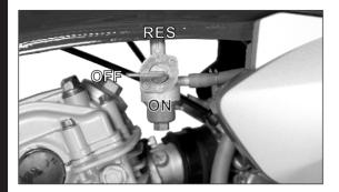
While riding with fuel cock lever in 'ON' position and if the fuel in the tank reaches reserve level, you may experience engine sluggishness and jerky feeling. Take the vehicle to the left side of the road while taking care of traffic and change the fuel cock lever position to 'RES'.
