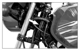
The frame serial number is stamped on the left side of the steering head tube.
