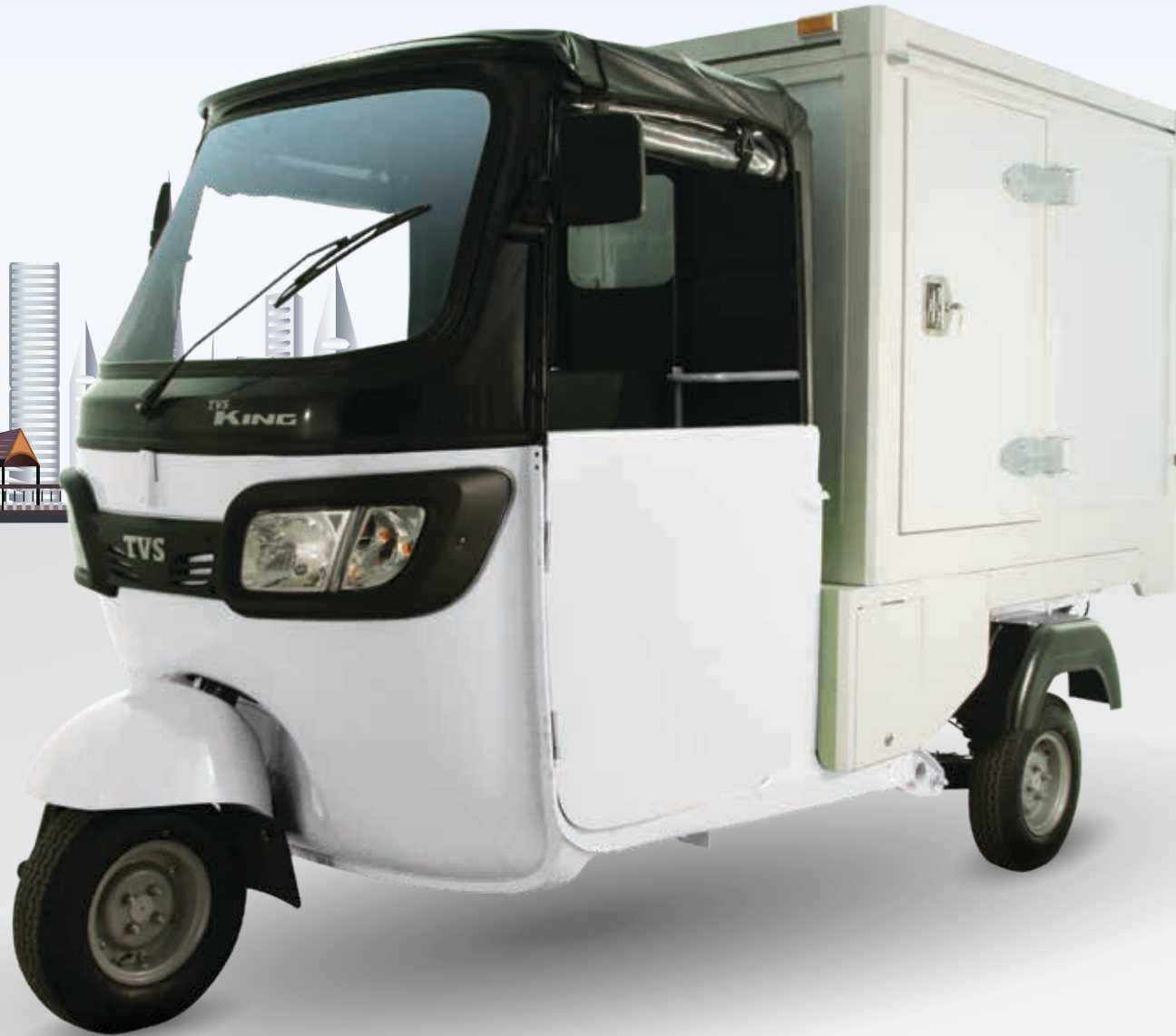
TVS KARGO BOX attachment dimension 1400mm x 1300mm x 1060mm
