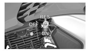
Fuel cock is located on fuel tank at the left side of the vehicle. Fuel cock has the following three positions,
