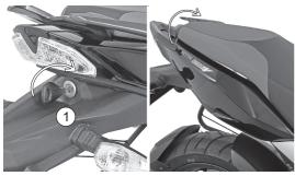
The seat lock (1) is located at the rear end of the vehicle bellow the tail lamp assembly.
