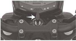
The engine can be started. The key cannot be taken out from the lock.
