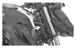
Frame serial number is engraved on the right side of the steering head tube as shown in the above figure.
