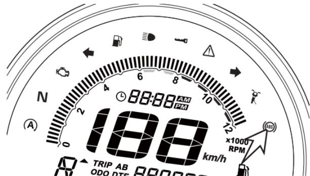
The TVS RONIN does an automatic self check every time whenever the ignition lock of the bike is turned 'ON'. The ABS warning lamp provided on the instrument cluster blinks and informs you that the ABS is under check.
