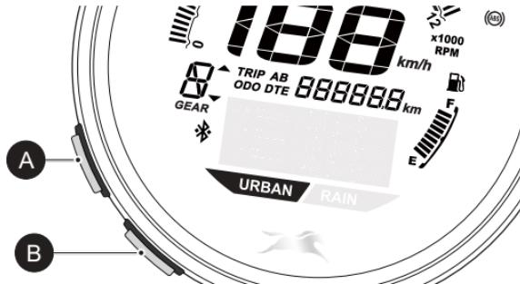
The 'Mode' (A) and 'Set' (B) buttons are provided to change between various modes and to set the some of the digital display functions of the instrument cluster. The sequence of modes and their selections are explained in detail below.
