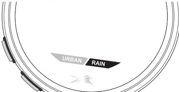
In 'Rain' mode the ABS braking system is modified to suit wet or rainy condition. The ABS intervention is earlier and safe braking will be felt.
