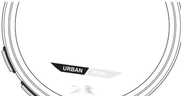
In 'Urban' mode the ABS braking system is modified to suit city on all types of roads riding condition. The ABS braking system is optimized accordingly.
