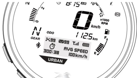
Once the cluster is connected with the smart phone the cluster displays the signal strength of the network provider 'Signal' (depending on OS version) and the battery level 'Battery' of the smart phone. Number of unread messages '✉ 6' for that particular ride and number of missed calls '📞 5' for that particular ride.
