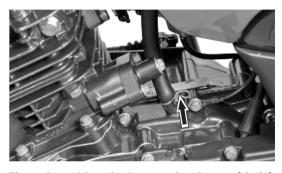
The engine serial number is stamped on the top of the left side crankcase near cylinder block.
