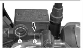
If the brake fluid level is below the mark or while applying brake if you feel the brake is more spongy or ineffective due to air entry, contact TVS Motor Company Authorised Distributor or Dealer / Authorised Service Centers for topping-up the brake fluid, air bleeding and other brake related inspections.
