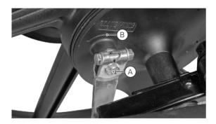
Incase the mark is going beyond the wear limit, index the lever to next slot with the help of Dealer to extend shoe life.
