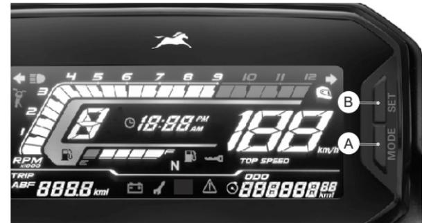
The Mode (A) and Set (B) buttons are provided to change between various modes and to set some of the digital display functions of the instrument cluster. The sequence of modes and their selections are explained in detail below.
