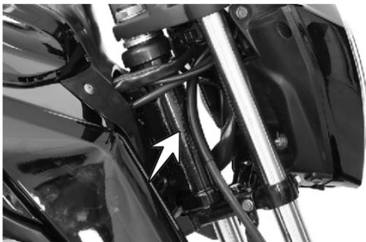
The frame serial number is stamped on the right side of the steering head tube.
