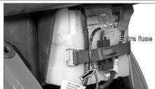
Inspect the fuse for failure. If found defective, replace the fuse (extra fuse is provided in the wiring harness itself).
