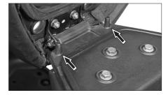
Two helmet hooks are provided under the seat assembly at front end near the seat hinge to secure your helmet. Open the seat assembly (refer page no. 25) to access the helmet hooks. Hook the helmet strap in the helmet hook properly and close the seat assembly.
