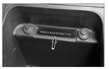
The frame serial number is stamped on the frame, at the rear end below the seat assembly. Open the seat assembly to read the frame number.
