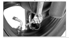
Brake shoe wear indicator (Drum brake)
