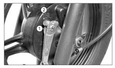
In case the wear limit index mark (1) is going beyond wear limit indicator (2), index the lever to next slot with the help of Dealer to extend shoe life.
