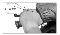
If the measured distance is more than the limit, adjust the nut provided at the rear wheel end to obtain the correct play.
