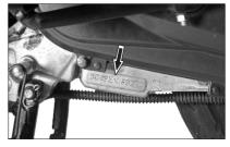
The engine serial number is stamped on the left side of the engine, at bottom, near centre stand mounting. See bottom to read serial number.
