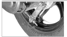
Turn the adjuster nut in clockwise direction for reducing free play or in anti-clockwise direction for increasing the free play.
