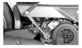
The kickstarter lever is located on the right side of the engine. The engine can be started by kicking the lever with the ignition key in 'ON' position while applying the rear brake as a safety precaution.
