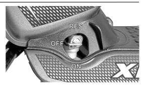
While riding the vehicle with fuel cock lever in 'ON' position and if the fuel in the tank reaches reserve level, you may experience engine sluggishness and jerky feeling. Take the vehicle to the left side of the road while taking care of traffic and change the fuel cock lever position to 'RES'.
