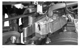
The engine serial number is stamped on the top surface of right side crankcase near engine breather tube.
