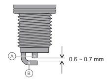
Inspect the spark plug electrodes (A) and (B) for any corrosion. If found any, replace the spark plug with a new.
