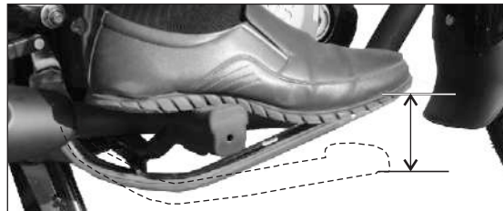
Checking rear brake pedal free play
