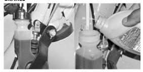
Brake fluid level checking & topping up
