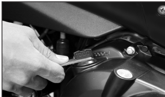
Open end to open & tighten dipstick oil.
