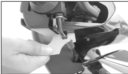
Open end to adjust throttle cable play.
