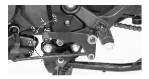
TVS STRYKER 3V is equipped with a 5 speed constant mesh transmission. Neutral (N) position of the transmission is indicated by the warning light on the speedometer.
