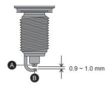
Inspect the spark plug gap. The gap should be 0.9 to 1.0 mm. If the gap is found to be more than the limit replace the spark plug with a new one.
